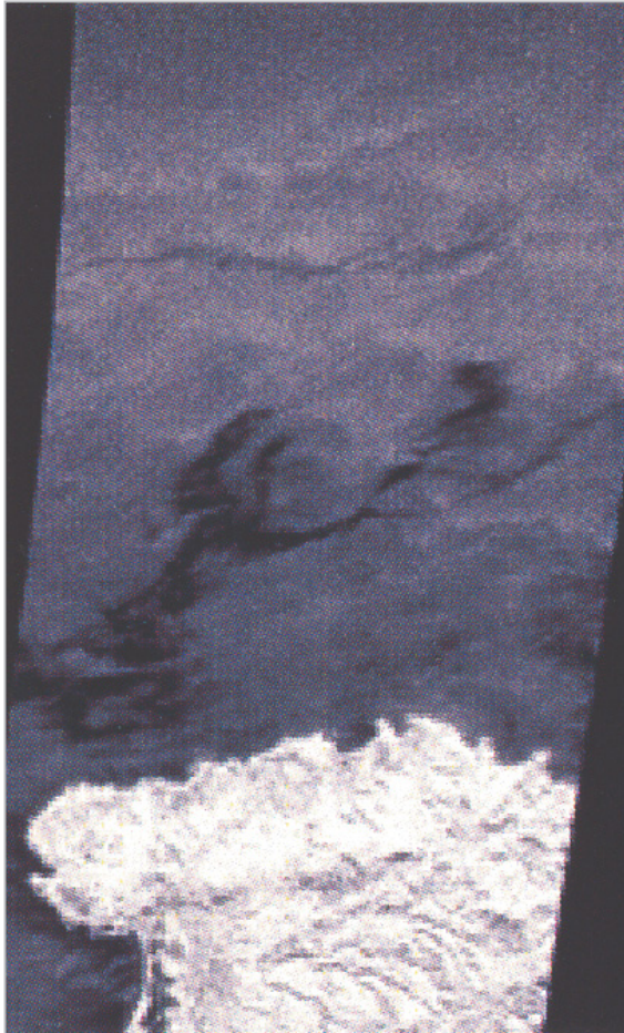
Fig.16 Image of crude oil spilled from Nakhodka tanker (L-band, VV polarization, off the coast of Noto Peninsula)
